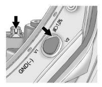
Locate the vertical headlamp adjusters, which are under the hood near each headlamp assembly.
